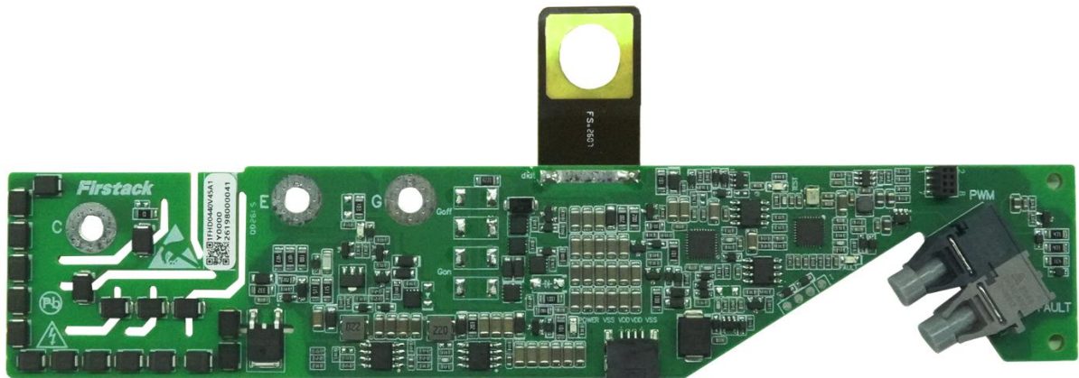
Fig.1 1FHD0440(including reeds required for the di/dt protection)
