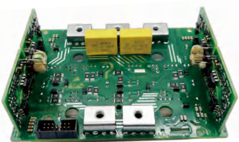
Two IGBTs in parallel installation unevenness <50um
