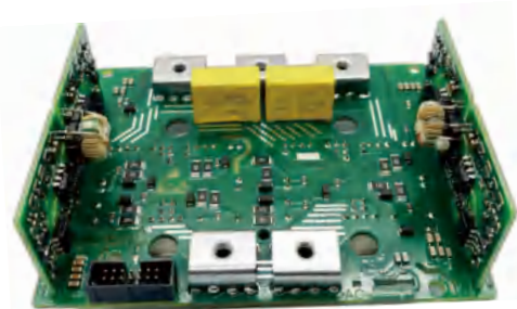
Two IGBTs in parallel installation unevenness <50um
